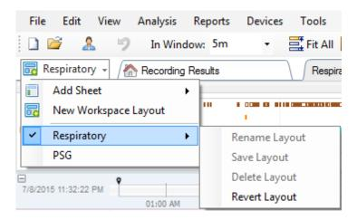
To save a customized signal sheet you right click on the signal sheet tab and select **Save Sheet Layout As...** When you have saved the customized signal sheet you can always **Update Saved Layout** if additional changes are made. For further information on signal sheets refer to the *Signal Sheets* section.
