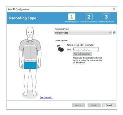
If your Recording Type is set up to record data from an auxiliary Bluetooth device, e.g. pulse oximeter you will see that in the Configuration Wizard. To be able to use auxiliary Bluetooth device it needs to be paired to the Nox recording device. Enter the appropriate Bluetooth device Pin/BDA (Bluetooth Device Address) number in the relevant field in the Configuration Wizard.
