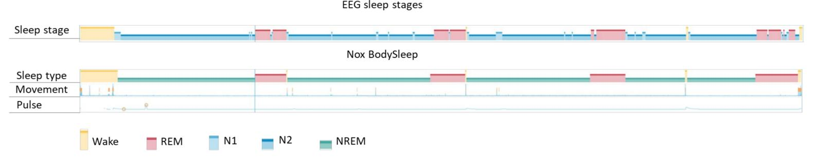
An example showing the comparison of the sleep type estimation of the Nox BodySleep and sleep stage scoring from EEG in a patient with a pacemaker where the pulse is stable around 50 BPM.
