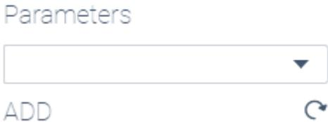
The order of the parameters can be changed by dragging the parameter labels, they can be removed by right-clicking on the label and selecting DELETE and as well as setting what parameter is a REFERENCE parameter. Setting the reference parameter will freeze that single parameter while scrolling through the records library.
