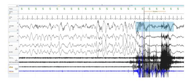
The below example features an abrupt change in EEG frequency and amplitude and increased EMG (EOG) consistent with REM arousal.
