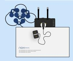
Secure the Nox A1s set-up sheet by attaching the Nox Abdomen Cable connector cable onto the Nox A1s recorder. Make sure the cable extends downwards from the recorder as per usual installation.
