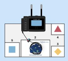
Attach the Nox SAS Head cable to the Nox A1s. Bundle the Nox SAS Head Cable connector to fit into the green circle pocket. Leave out the connector for the two Nox SAS body cables so these can be connected in a later step.
