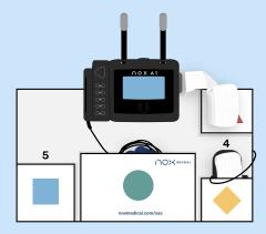
Prepare the abdomen RIP belt by attaching one end of the RIP belt to the connector. Wrap the white belt around the abdomen connector and store in the yellow diamond pocket.
