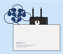
Configure the Nox A1s for SAS and insert a fresh or fully charged battery.
