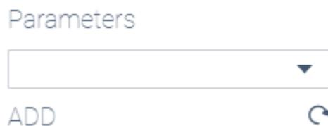
The order of the parameters can be changed by dragging the parameter labels. They can also be reordered with arrows by right-clicking on the label and selecting “REORDER WITH ARROWS.” They can be removed by right-clicking on the label and selecting DELETE. You can also set what parameter is a REFERENCE parameter. Setting the reference parameter will freeze that single parameter while scrolling through the records library.
